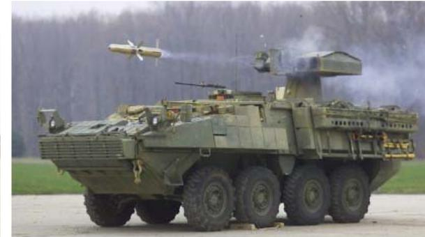
*M1134 Stryker Anti-Tank Guided Missile. The ATGM variant is intended to provide a highly mobile anti-tank capability, using a remote control turret with sensors and a pair of TOW missile launcher tubes. The system is intended to supplement the MGS.*
