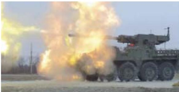
*M1128 Stryker Mobile Gun System. The Stryker brigades will derive much of their fire power from the MGS system, which is equipped with a 105mm gun common to early variants of the M1 Abrams tank. The MGS has a stabilised turret, permitting the three-man crew to fire on the move.*
